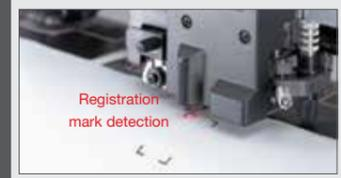
By continuously detecting a maximum of 4 register marks nested images in both X and Y axis direction can be cut aligning each image automatically. Detecting one register mark is sufficient when using Mimaki's FineCut software.
